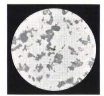
UNDISPERSED Cement in water in its normal flocculated condition. Photomicrographs — Magnification 300
