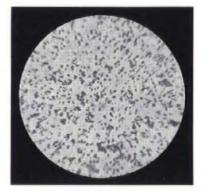
DISPERSED Cement in the dispersed condition produced by adding a dispersing agent.
