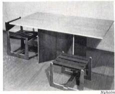
The table and resin-bonded plywood sheet at the The table and resin-bonded plywood sheet at the right illustrate the essential simplicity of Cog-geshall's method. The table was made entirely out of a similar sheet of plywood, its cost being little more than the cost of the stock. No glue is used in any of the pieces, and the screws serve merely to hold the structural members in place. Above, a folding dining table, canvas-webbed chairs, book-case, and a desk with removable top.
