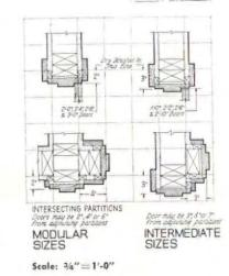
**DOORS** of all standard sizes are adapted to modular planning by the use of appropriate details. Modular sizes (4 in. multiples) should be placed 2 in. from the coordinates, intermediate sizes 3 in. from this line. Table shows relationship to stud spacing.
