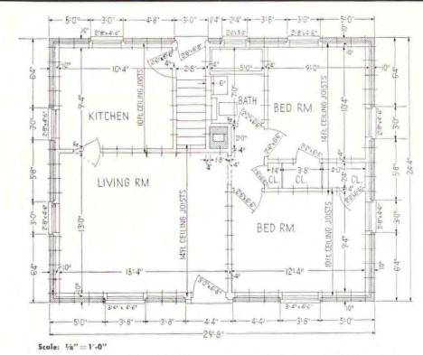
APPLICATION of modular planning principles to a typical low cost house. All dimensions are multiples of 4 inches; stud centerlines show how framing has been taken into account in locating partitions and door and window openings.
