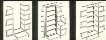
Leave opening in back wall Set ventilator in place Lay up front wall—and that's all.
