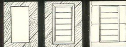
Cut opening in sheathing Nail ventilator in place Butt siding against body—and that's all
