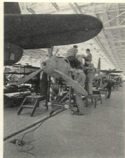
Drag chain conveyor recessed in the floor parallel to the production line pulls the fuselage jig from station to station at the rate of 2 ft. per hour. Note power outlet electricity and compressed air; there is one every 15 ft. down the line.
