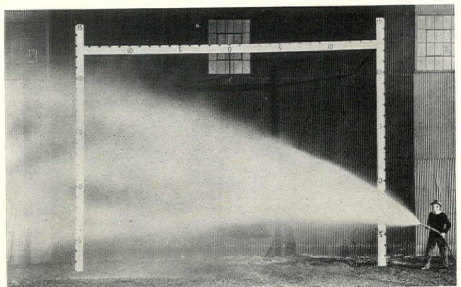
A WATERFOG rather than a water stream comes at high speed from this specially designed hose nozzle, thus permitting fires
