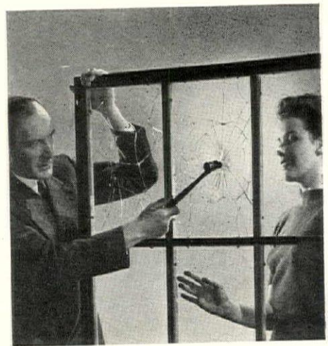
BROKEN GLASS , biggest civilian hazard in wartime, is held safely intact by a transparent film applied to inside window surfaces in the form of a quick-drying liquid (p. 58)
