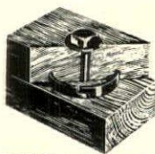
TECO Ring Connectors spread the load on a timber joint over practically the entire
