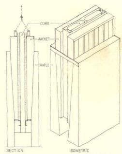
Improved casting apparatus, which Mr. Atterbury has recently developed, utilizes a light, inexpensive "jacket" supported in a cradle strong enough to resist the hydraulic pressure of the 8 ft. casting. Jacket can be removed after concrete has received its initial set, freeing cradle for another casting.
