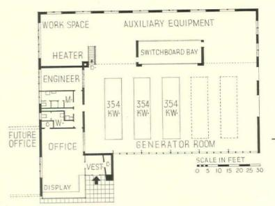
The Border Counties Cooperative is located in Warroad, Minnesota, near the Canadian border. It is the most recently completed REA generating plant. Placing of the storage area at the rear permits future expansion of the generator room. As in the Tri-County plant (page 81) the generating room is also used as a display feature. Architect, engineer and contractor: General Engineering Corporation.
