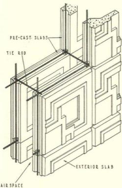
Above, right, Millard house, Pasedena, Calif., best known of the structures by Frank Lloyd Wright employing his "Textile Block" method of construction, developed in 1921. Details above show relief pattern in face of block and method of assembling double, hollow walls and joining the units with a "warp and woof" of steel reenforcing bars grouted into the joints.
