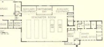
The Tri-County building, in Portland, Michigan, is a combined diesel generating plant and office headquarters. Its main element, the generating room, has been treated as a display feature, from both inside and outside the building. The customary offices for a distribution cooperative are located in the right end of the building. Note the accordion partition between lobby and meeting room, giving excellent flexibility in the use of these spaces. Architect and Engineer: J. & G. Daverman Company.
