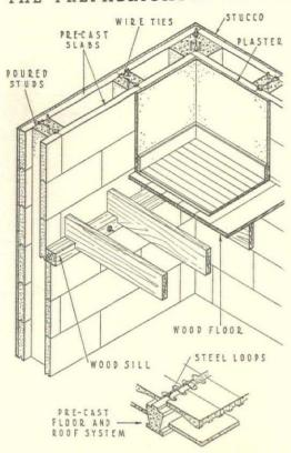
Above, Hahn system of construction from precast concrete "lumber," used in Illinois and Wisconsin in 1919. Below, Knapp Unit Wall construction, now being extensively employed in California.
