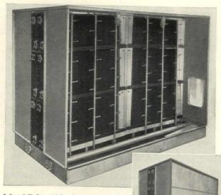
(above) Dehumidifier (air intake side) Unit consists of a sheet metal enclosure housing from 4 to 24 Modine Steel Cooling Coils (depending on size of unit). On inlet side of coils a series of nozzles spray water over the coils.
