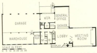
The Burt County headquarters, at Tekamah, Nebraska, is built of reenforced concrete. Its layout is considered by REA as one of the best yet developed. Especially workable features are the lobby and meeting room, used separately or together, and the manager's office, which overlooks both garage and general office. Architect: H. H. Henningson Engineering Co., Inc.
