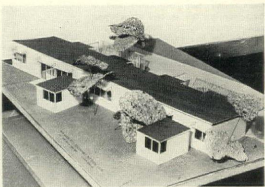
ONE-STORY ROW HOUSE designed by H. McK. Jones. The model shows the garden side, with the additional, transportable bedrooms projecting from two of the dwelling units. Accommodations consist of living, dining, kitchen, bathroom and utility space plus a permanent bedroom unit, apart from the transportable one.
