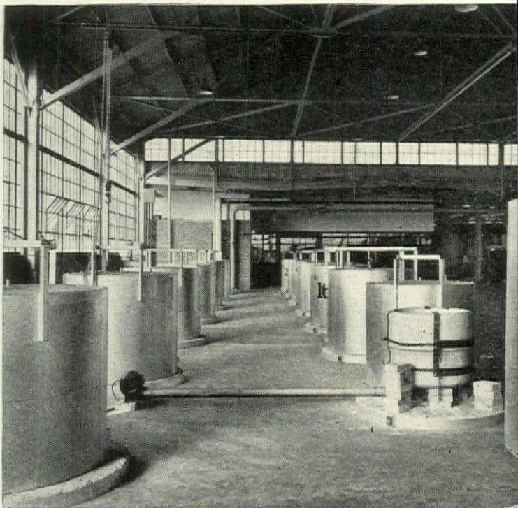
INTO THESE KILNS the pots of molten glass are set for cooling after the melting operation. Because the glass will finally be used for very precise optical lenses, great care must be taken in controlling every step in the manufacture. Temperatures must be very rigidly checked.
