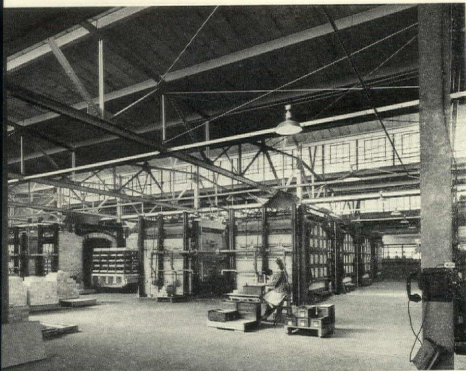
A GENERAL VIEW of the plant showing furnaces used in the second melting operation. Glass is placed on trucks which roll in and out of the furnaces on rails. In foreground an inspection is under way. A feature included in the design of the building is the window sash in the monitor of the building. This sash may be opened when necessary.
