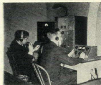
CONTROL PANELS include the amplifiers and regulatory equipment for the two channel system.
