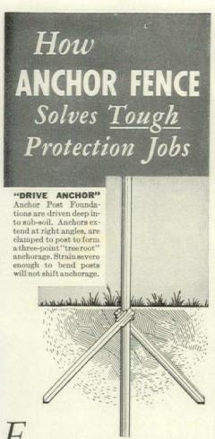
Rom Maine to California, architects have specified Anchor Fence for tough war plant protection jobs. They've counted on Anchor's exclusive features to give them faster fence erecting, greater strength, easier moving when necessary.
