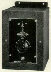
Shown above is the small Control Cabinet of a Webster EH-10 Moderator System, central heat control of the pulsating flow type. It can be used to automatically operate a motorized valve in steam mains, or directly control burner or stoker of your boiler.
