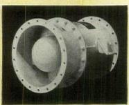
Marine type axial-flow fan 15%" in diameter; delivering 2000 CFM at 3" static pressure.
