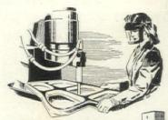
Peak welding efficiency is made possible by cooling of welding tips with water or brine held at the right temperature.
