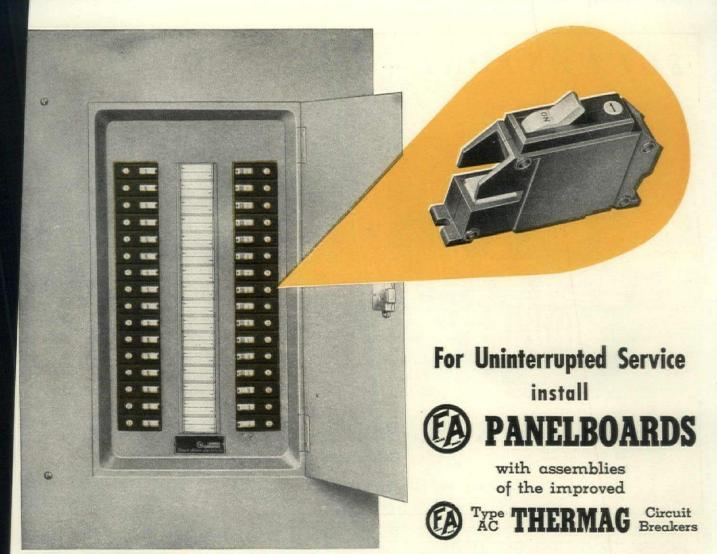
The Safety Panelboard above is Catalog No. (A) NACIB32-3L20 It contains 32 (B) Type AC Thermag Circuit Breakers, and 200 ampere 3 wire main connection. An enlarged view of the individual Circuit Breaker is shown at the right.
