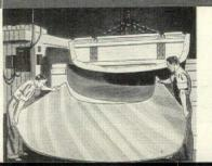
There are several methods of producing molded plywood shapes bonded with BAKELITE Phenol Resin Glue. Essentially, all of them involve the laying up of veneers in diagonal strips over or within a form, after which low fluid pressure and controlled temperatures are applied, which force the plywood assembly to the exact contour of
