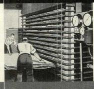
Thin veneers of wood are spread with BAKELITE Urea Resin Glue, then assembled with each adjacent layer at cross grain. This assembly is pressed to a smooth, strong plywood panel. To save production time, many manufacturers use a hot press, to form the panel under both heat and pressure.
