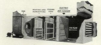
Cross section of Precipitron installation in typical air conditioning duct.
