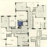
EXTRA APARTMENT per floor is made possible through using a mechanically ventilated bath in center of the building.
