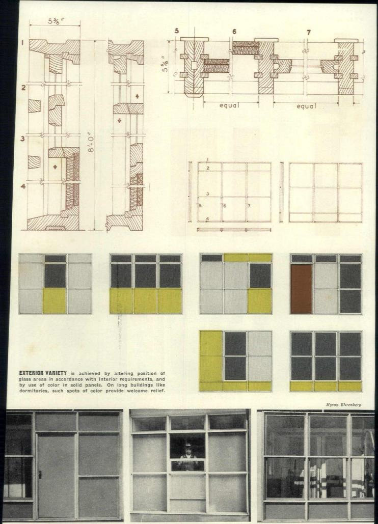
PANELS PROVIDE MINIMUM AND MAXIMUM GLASS WITH EASE. SASH SLIDE IN FRONT OF SOLID SECTIONS
