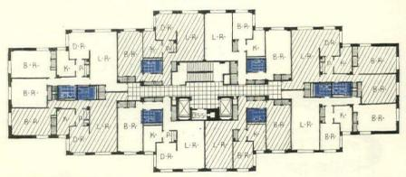
LAYOUT ADVANTAGES of the inside bath can be noted in this apartment plan for the Equitable Life Assurance Society. By locating baths in interior parts of the building, larger window area can be achieved in other rooms.
