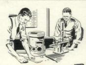
Super accuracy in gauge rooms is possible when the air is clean, dehumidified, and maintained at a constant temperature.
