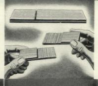
Plywood bonded with BAKELITH Urea Resin Glue is recommended for practically any interior use. I has good "wet-strength" and excel lent "dry-strength." It is extremely low in cost, yet the bond is strong or than the wood itself, and remains so even though the plywood panel is subjected to long period at high humidity.
