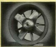
All aluminum Aviation type axial-flow fan. 70 lbs. complete with 2½ HP motor; 4300 CFM at 2" static pressure.
