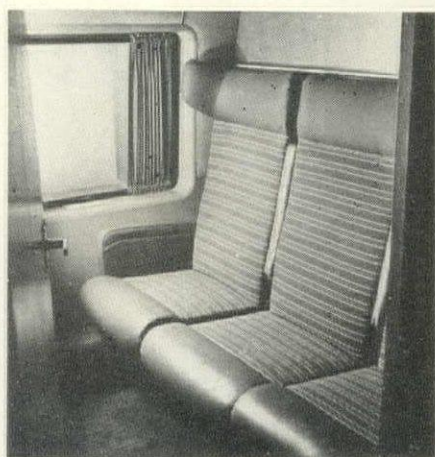
SEATS RECLINE, END TIER BECOMES A PRIVATE COMPARTMENT WHEN PARTITIONS EMERGE FROM SEAT BACKS AND WALL
