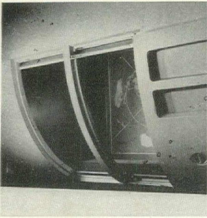
WHEN HORIZONTALLY SLIDING ENTRANCE DOORS CLOSE, TWO LOUNGE SEATS FOLD DOWN FROM RECESSED PANEL
