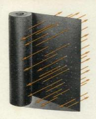
Pin-point perforations form "Inlet" and "Outlet" Valves . . . vapor escapes through perforations and so prevents roofs from blistering and buckling.
