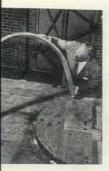
upon cooling, the urea wood is its newly acquired shape. are two types of urea wood: noplastic and thermosetting.
