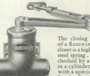
The closing power of a Russwin doorcloser is a high-grade steel spring ... it is checked by a piston in a cylinder filled with a special nonfreezing liquid.
