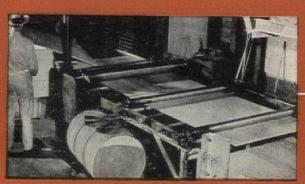
panels. This is a flood-spreader type of machine for the applica-tion of Laucks plywood treating solutions.
