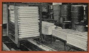
A mono-rail basket in operation. Materials to be treated are carried in a weighted cage and "dunked" in Laucks preservative water-repellents. This type of tank is generally used for the treat-ment of sash, doors, etc.
