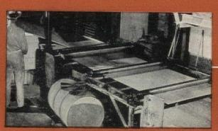
In most plywood mills a Reziting machine is used to treat panels. This is a flood-spreader type of machine for the application of Laucks plywood treating solutions.
