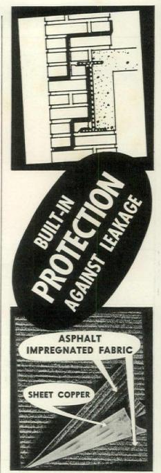
Slick-surfaced metal flashing is slippedin protection against leakage. WASCO rough, fabric surfaced, sheet-copper centered flashing is built-in protection against leakage. The impregnated fabric forms a perfect bond with the mortar, free of seepage-inviting, hair-line cracks. Electrolysis will not destroy its sheet-copper center because the impregnated fabric and asphalt binder are effective insulation against electrolytic action. May we send our A.I.A. folder?
