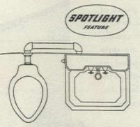
THE DRESSETTE FLOOR PLAN Right or left-hand installations provided. The Junior Dressette offers spacesaving features for the small bathroom or powder room. The Eljer Dressette combines a high-quality and modernly designed lavatory and closet in an efficient unit ... an Eljer spotlight feature that gives profitable distinction to your bathroom planning and building.
