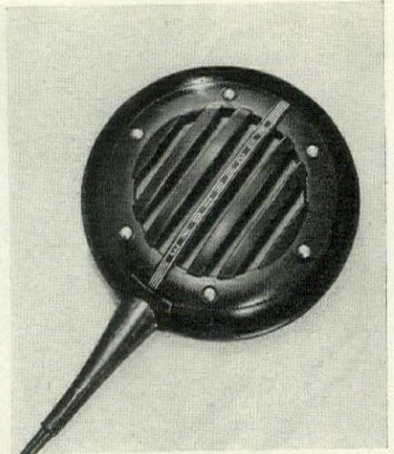
tension speaker for individual listening. Its flat disc shape, 4 3/16 in. by 11/16 in., makes it ideal for under pillow use in bed. Hermetically sealed it can be cleaned in disinfecting solutions not over 120° F. A light weight "Bimorph" crystal element insures uniform response and high sensitivity. Its tone quality is comparable to large cone-type speakers, and it produces sufficient volume with only .01 w. power consumption.
