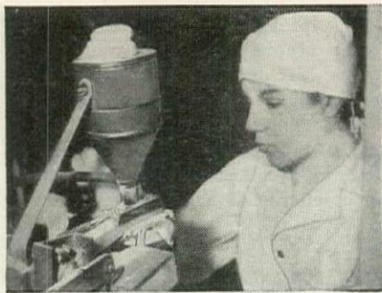
2. Starting growth of Penicillin. In this small, sterilized and enclosed room, the operator feeds powdered Penicillin culture into the flasks containing a corn starch base mixture. The flasks are then sent to the incubation room.
