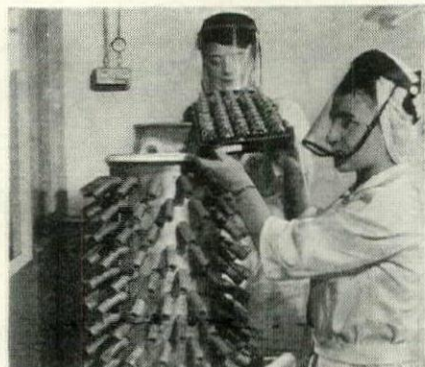
5. Sealing Room, where small bottles of liquid Penicillin are sealed after removal from the refrigeration room. They are now ready for shipment. The sealing room is maintained at constant temperature by the Honeywell thermostat at upper left.
