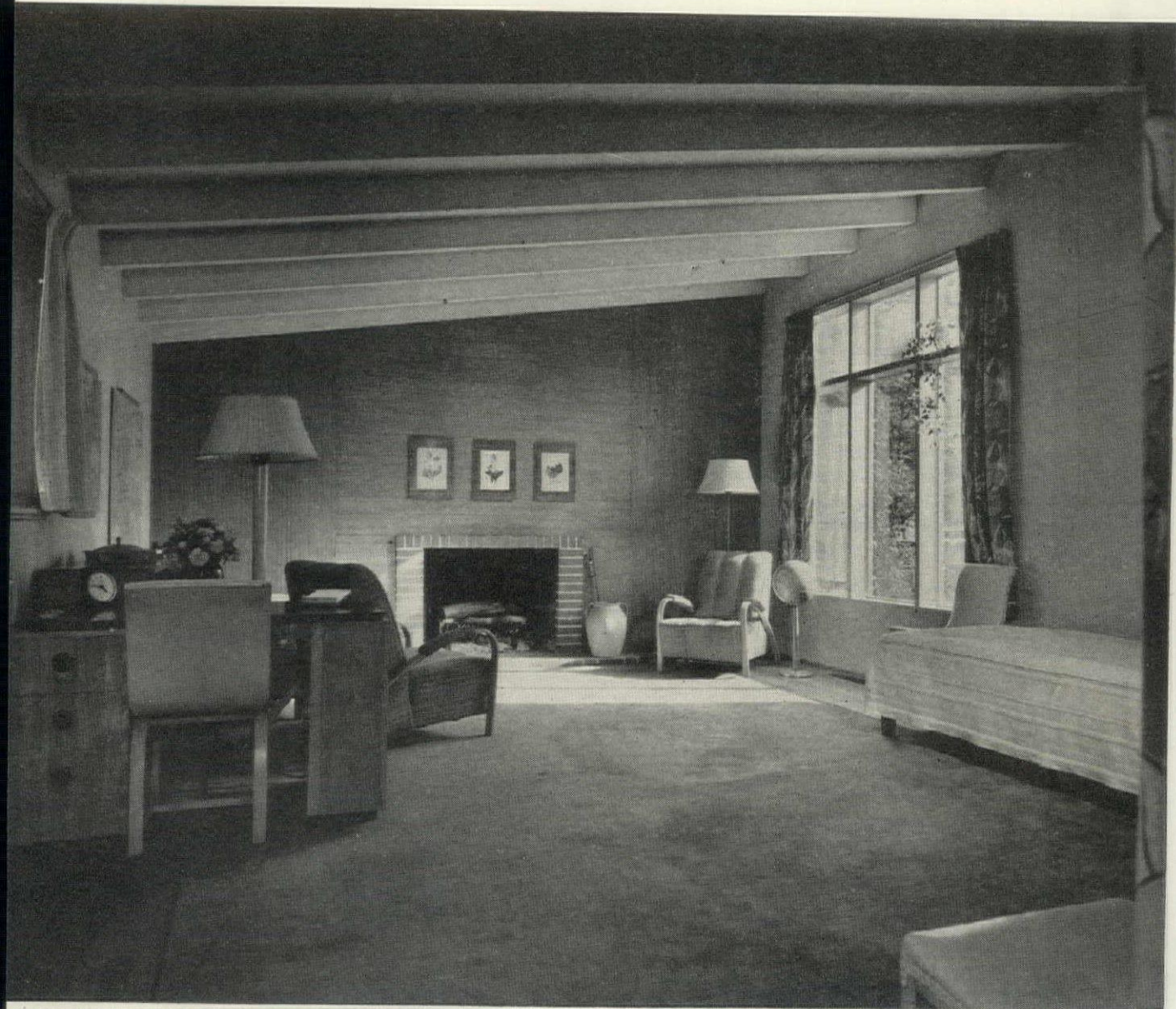
G ROOM HAS THE HIGH SIDE OF SHED ROOF ON SOUTH TO ADMIT MAXIMUM SUNSHINE. NOTE EXPOSED RAFTERS
