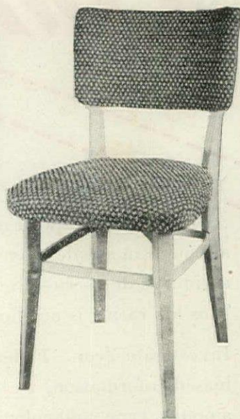
DINING CHAIR is best designed item. Diagonally opposite front and back legs and back support are factory joined in a flat piece. Two such sections, assembled in an X, form the frame.
