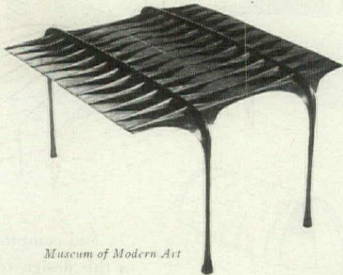
The design principle of the lily pad—a system of rods and membranes in tension—has important implications for metal construction, as evidenced by this welded structure by Paul Nelson.
