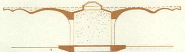
Although a ripple formed the basis of his design, Workman's concrete shell—40 ft. across, 2 in. thick at edge—shows the practicality of the principle.
