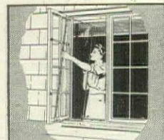
DUAL GLAZING —a single panel type that mounts on inside of sash. Inconspicuous. Easily removed for cleaning.
