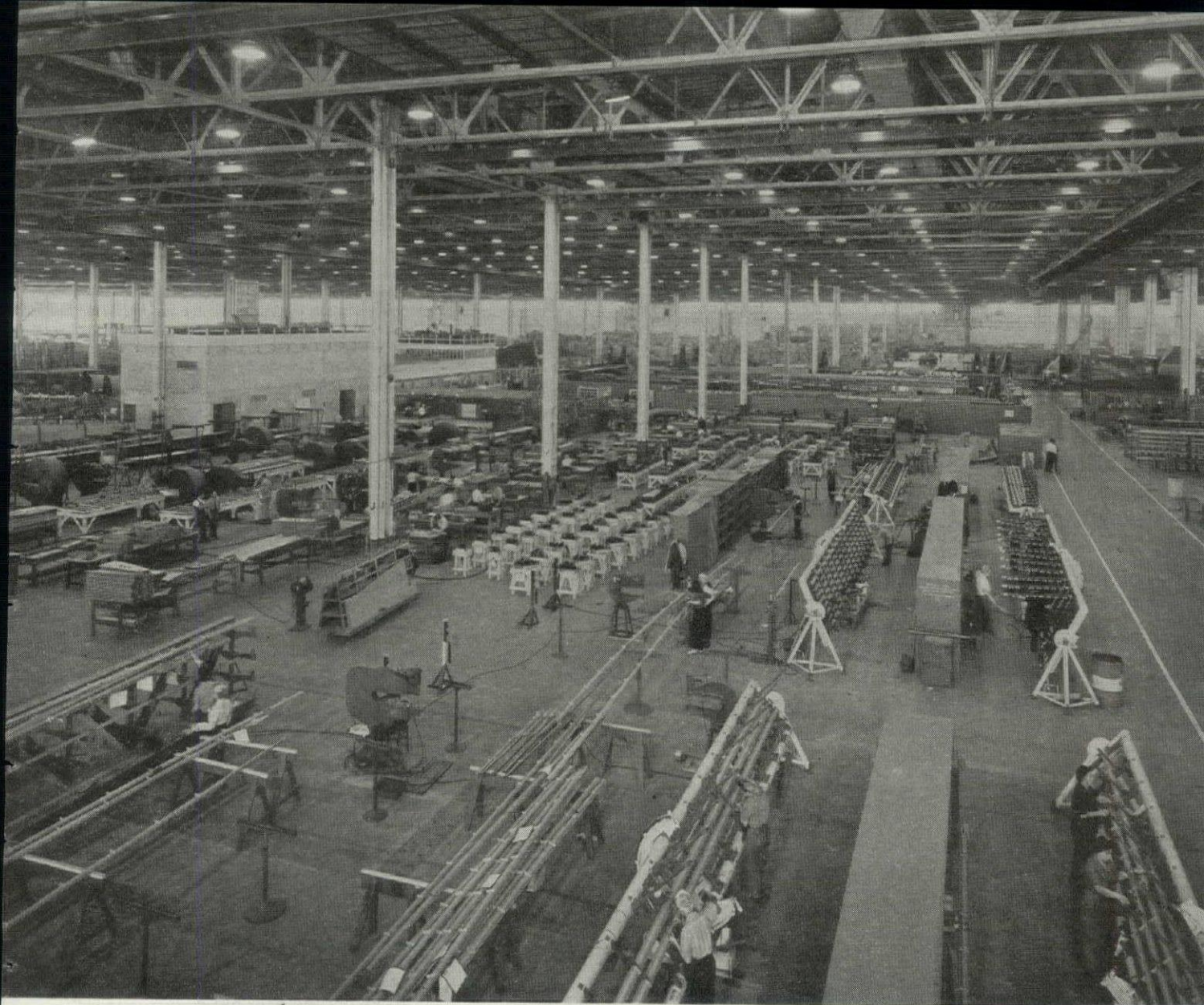
MANUFACTURING AND SUBASSEMBLY AREA OF MAIN PLANT. NOTE ONE OF TOILET AND CANTEEN ISLANDS, CENTER LEFT
