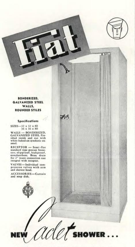
Redesigned along modern lines with improved construction features. The Fiat tension locking joint is used on all four corners and in joining the side walls with the receptor. No screws are used in any of these joints. This construction speeds erection on the job and assures a watertight shower cabinet with unusual strength and rigidity.
