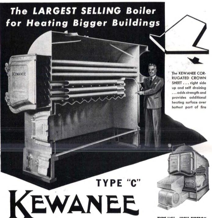
The Sawed-in-Two Type "C" Kewanee pictured above indicates why it has become the largest selling boiler for heating big buildings. Note especially the corrugated Crown Sheet, for extra strength and heating surface . . . the big, high firebox . . . the long travel of gases . . . and the ample water content and plenty of steam space. Over-all efficiencies of 80% and more are not uncommon with this fast steaming boiler.
