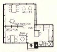
TYPE IC is a conventionally-built branch library consisting of three rooms, and accommodating 3,000 books. Interior sketches show conversion of unit for motion pictures and meetings. Sectional shelving forming partition can be taken down in a few minutes.
