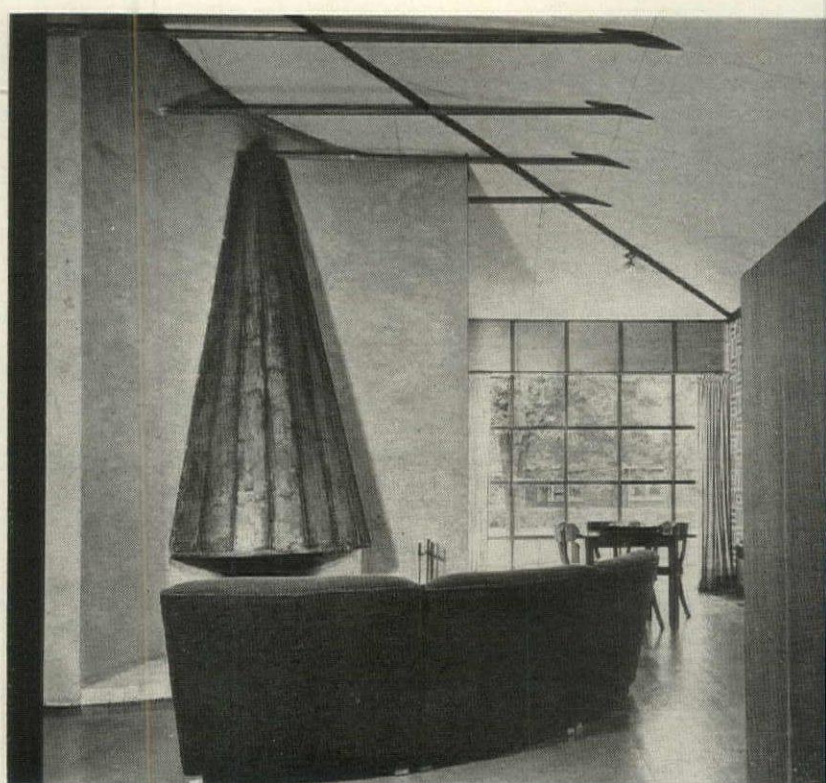
ROOF TIES RUN THROUGH FIREPLACE AND SHEETMETAL HOOD
