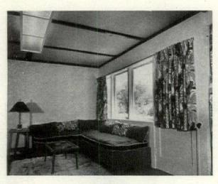
STANDARD BOX LIGHTING fixture is used on wallboard ceiling. Framing is exposed. Economical construction of window and door opening nevertheless produces a neat, simple appearance.
