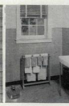
FABRIC COVERINGS are particularly suitable for finishing the dry-built walls of kitchens and bathrooms. They hide the joints in wallboards and provide a permanently washable surface. The material being installed in the photograph above is Sanitas, a product of Standard Coated Products Division of Interchemical Corp. It consists of 4 coats of paint baked on a strong fabric foundation and is available in plain colors, stripes and a variety of other patterns.
