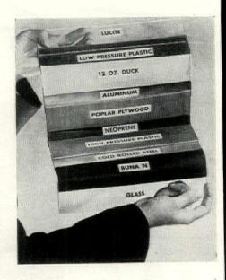
CHAIN OF MATERIALS is made with U. S. Plywood Corp's. "Pliobond" which its sponsor claims "bonds anything to anything." For most applications neither high pressure nor heat is needed. The quick-setting adhesive may be brushed, sprayed, spread or roller coated.
