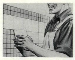
METAL TILE manufactured by Clyde (Ohio) Porcelain Steel Corp. weighs only 31/2 lbs. per sq. ft. and is quickly installed on a grooved foundation sheet which assures automatic tile alignment. One carpenter (not a tile-setter) can cover the entire walls of an average bathroom in a day, and the room will weigh a ton less than if finished with clay tile. Light weight framing may thus be used.
