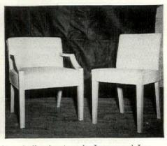
A SIMPLIFIED METHOD OF UPHOLSTERING employed in a new line of office furniture by Intramural, Inc. New York. Using U. S. Rubber's Kaylon webbi ng is first applied to the wooden chair frame and burlap stretched across the seat and back to make a foundation for the slabs of foam rubber. The seat and back cushions, precut to fit, are then cemented to the frame. With application of the outer fabric covering in the conventional manner, chair is completed.
