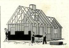
SHEATH OUTSIDE WALLS with Flintkote Asphalt Coated Sheathing. Efficient insulation plus ample structural strength. These large panels build fast as they insulate. Combine their double function of insulating and building, with the labor saving speed of installation ... and you get real economy.
