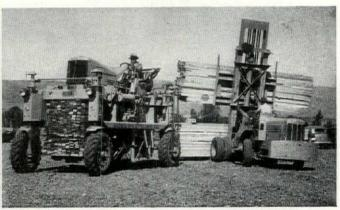
DITCHER AND LUMBER CARRIERS are specialized tools for large scale builders. The former, manufactured by Barber-Green Co., will dig pipe trenches for an entire subdivision in a matter of hours. The straddle carrier and lift truck are made by Ross Carrier Co.
