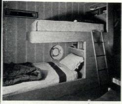
DOUBLE DECKED BUNKS offer a solution to the problem posed by small houses for big families. Here, Architect Edward D. Stone has staggered the bunks to permit a person to sit upright on either one.
