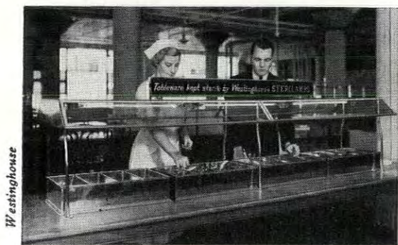
ULTRAVIOLET LAMPS , used over silver-, glass- and china-ware, are an important means of sterilizing, thereby reducing danger of infectious diseases such as trench mouth.
