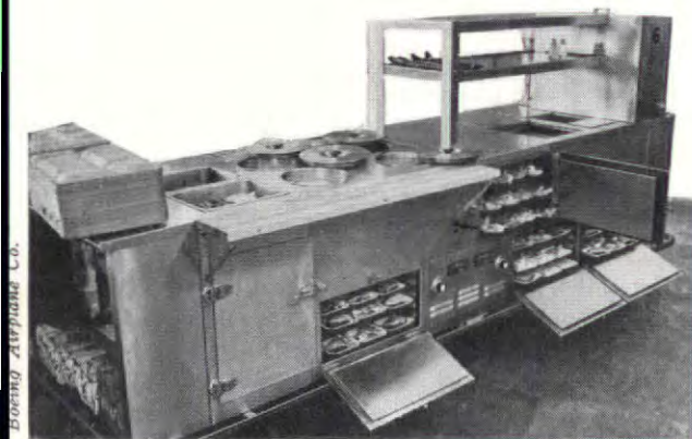
MOBILE FOOD CONVEYOR carries well-balanced meal of hot foods and soup, drinks, salads and desserts for 250 persons prepared in central kitchen. Various compartments are heavily insulated, electrically heated and cooled.
