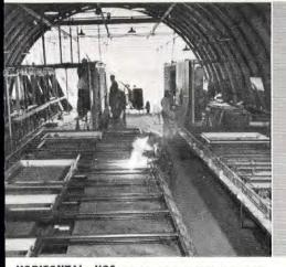
HORIZONTAL JIGS align subassemblies, containing steel window casings, with framing and bracing members. Center line produces rear walls; left, front walls; right, end walls.
