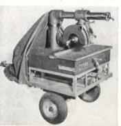
for fast, on-the-job cutting. By making the automatic precision cutting, versatility and production speed of this type saw available at the job, the Mobil-Shop increases manpower output, speeds construction, lowers costs. It allows power cutting to be done on the job that would otherwise be held up awaiting
