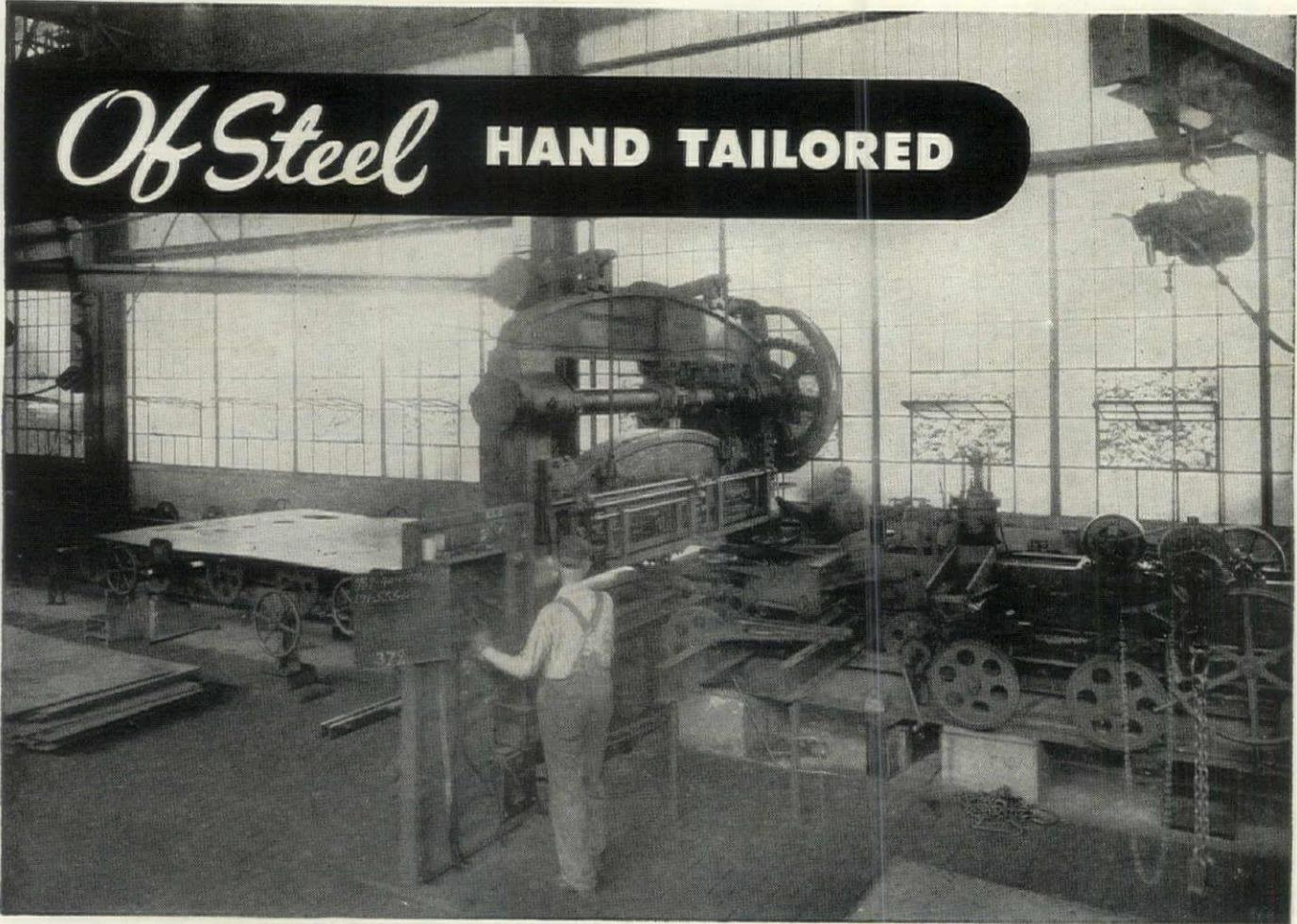
On these Spacing Machines, operated by skilled boiler-makers, rivet holes are "tailored" into heavy steel plate with an accuracy that's really uncanny.
