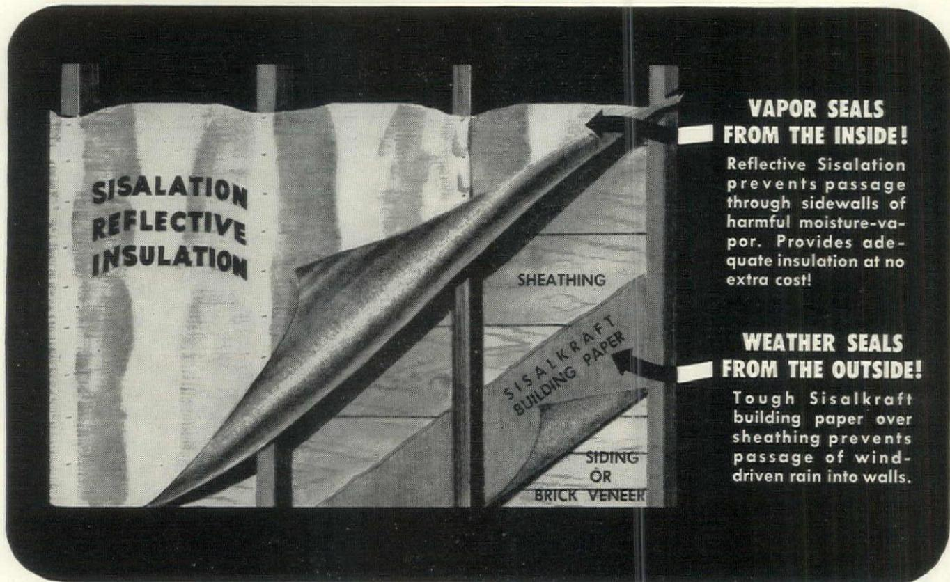
*See for Yourself:* New wall construction, utilizing the prime features of Sisalkraft and Sisalation, now enables you to stop the passage of harmful moisture into walls easily and economically. This simple method provides a permanent *dry wall* in homes PLUS all the advantages of adequate insulation at no extra cost! Write today for further information about these two products.
