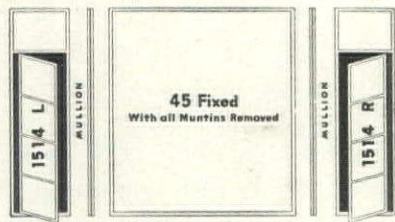
Remove all muntins from Ceco stock casement 45-Fixed. Combine windows with standard mullions.
