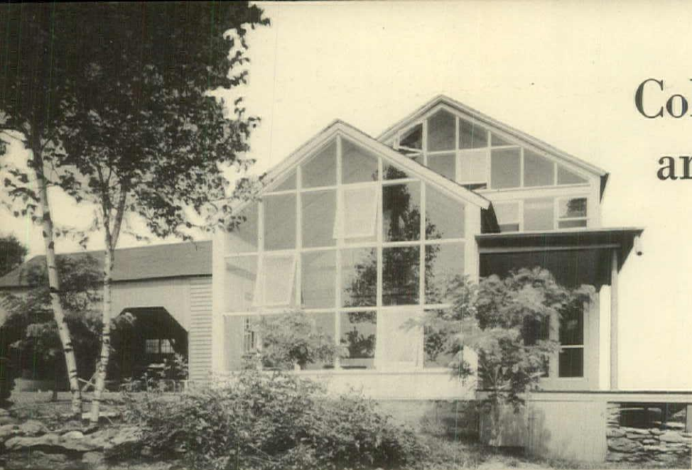
AWNING-TYPE WINDOWS, DEFTLY PLACED, MEET VENTILATION NEEDS ON THE SOUTH SIDE
