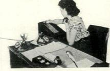
2. SALESMAN'S CODE SIGNAL is registered on the keyboard of the auto-sequence visual paging system. Six different calls may be flashed at the same time, in sequence, without loss of time in paging while calls are re-set, in the Wanamaker's installation. If ten successive digits are used for coding, 175 individuals can be called from the floor for conference.
