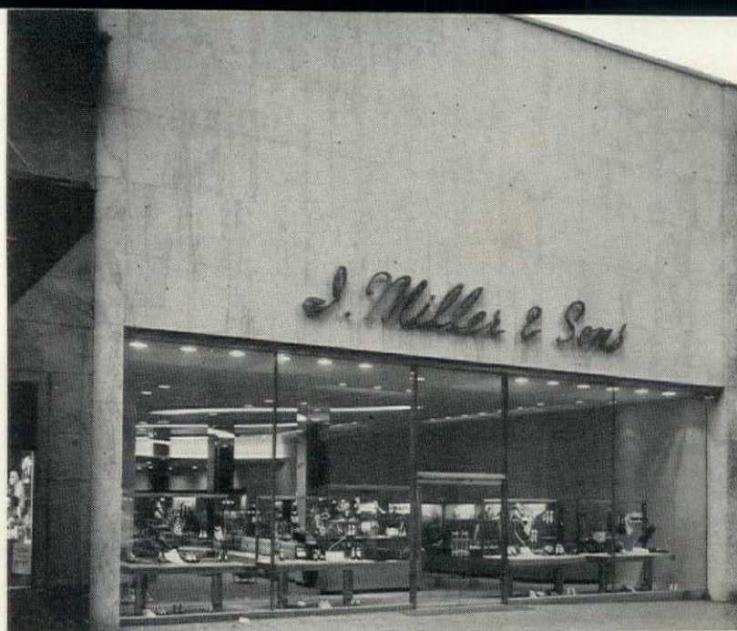
WHITE MARBLE FRONT HAS CONCEALED AWNING AT WINDOW HEAD
