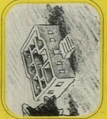
The traditional building will be erected in masonry construction of brick or stone, the only kind of heavy construction known when McGarkle Hall was built. Like the college's very first building, the new one will have heavy walls to support the load of floors and roof. Window openings must be narrow so not to weaken the load-bearing walls. And they must be placed so not to interrupt the symmetrical facade.
