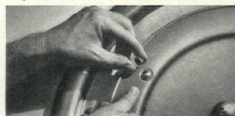
Step Two: Press "B" cone—slip out washers
