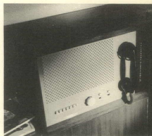
RADIO PANEL is perforated metal, accommodates light switches for trough and reading light, and telephone with handy, retracting cord. Radio switch selects six stations.
