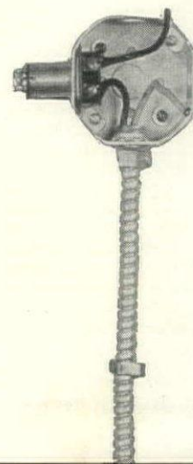
LOW VOLTAGE RELAYS shown inserted in switch boxes are the keys to the two systems. Square D's "Saflex" relay, above left, cuts regular house current of 110 volts to 24 volts. General Electric's "Remote Control" relay diminishes switching voltage to 25, mounts in cutout.
