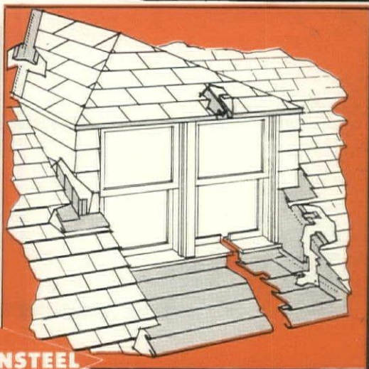
STAINLESS STEEL FLASHING for Dormer Window and Recess
