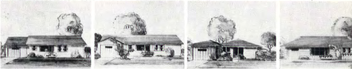
PLAN IS ROTATED, GARAGE SHIFTED AND ROOF VARIED TO PRODUCE FOUR DIFFERENT EXTERIORS
