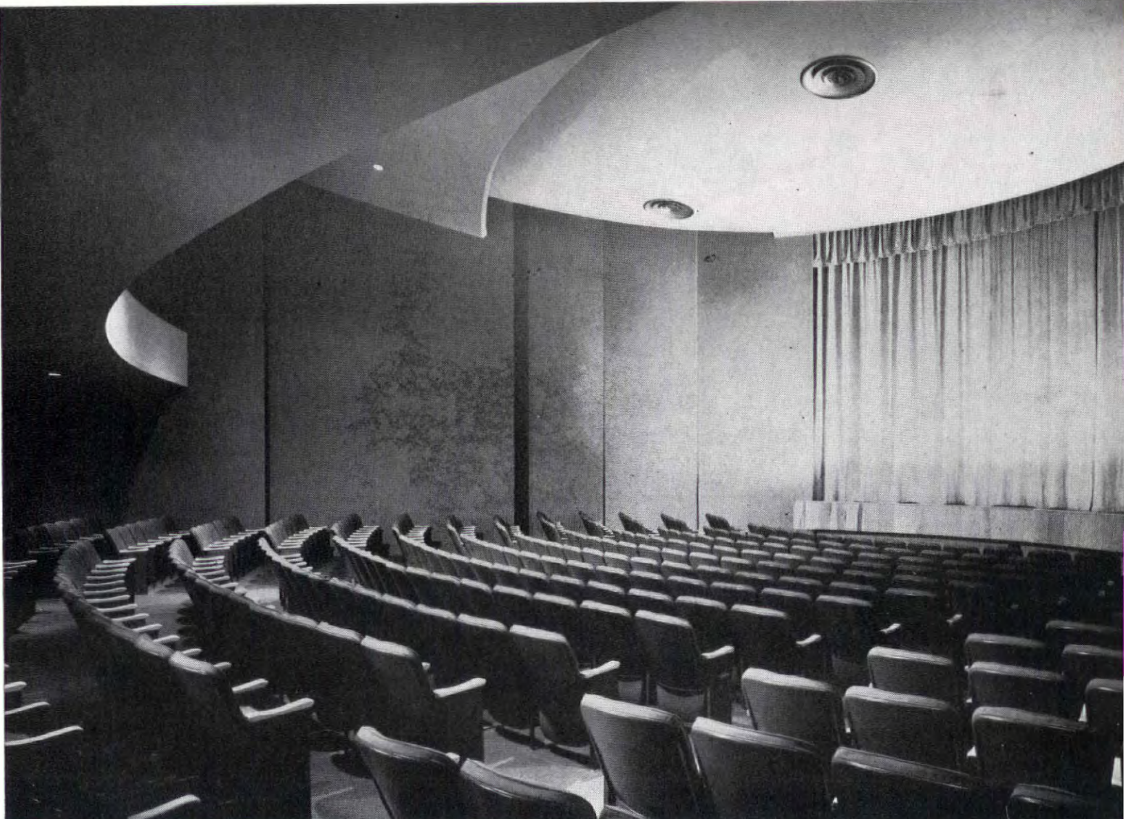
SERIES OF CURVES PROVIDES TOP VISUAL AND ACOUSTICAL PERFORMANCE. UPHOLSTERED SEATS ARE SPACED 35-40 IN. BETWEEN ROWS
