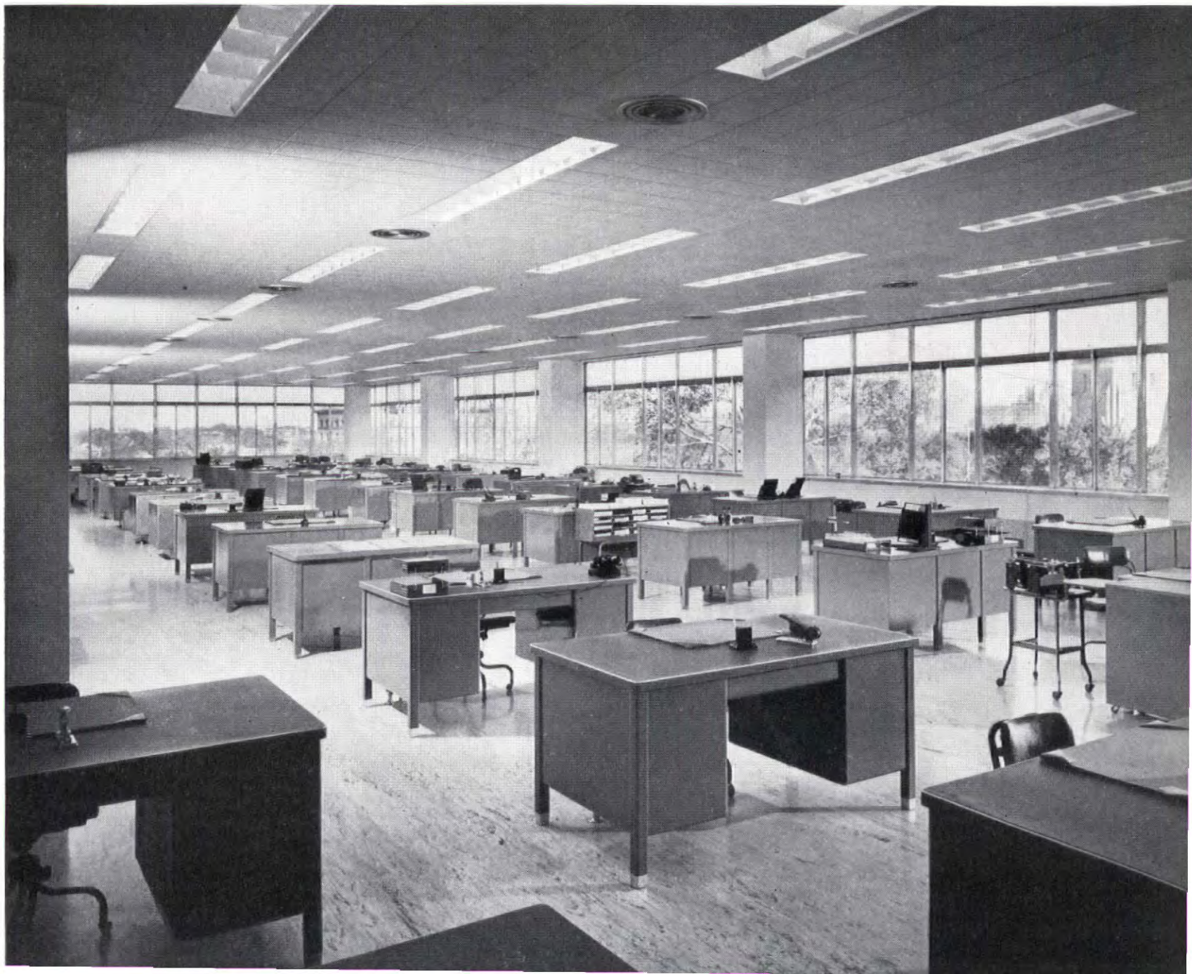
COOL AND WARM AIR ARE SENT INTO ROOMS THROUGH CEILING OUTLETS; CONVECTORS AT WINDOWS SUPPLEMENT AIR HEATING
