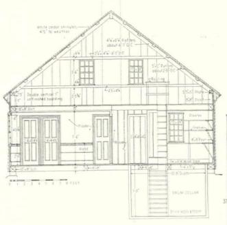
EARLY SECTION AND PLAN show typical construction features of the authentic Cape Cod: thin walls, shallow windows, low ceilings, no foundation, round brick root cellar and huge cooking fireplace with oven. Because it is a half house, the chimney block is placed off center to allow better room division. Stairs are thus in an atypical position, not braced against the chimney.
