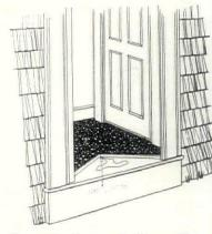
Grooved rain trough directs Cape storm water (which no door, however tight, could keep out) through floor to the sand below the house.
