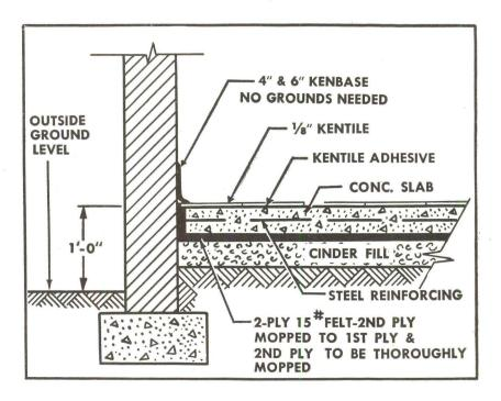
INSTALLS DIRECTLY ON CONCRETE. As shown above, Kentile can be installed on concrete in direct contact with the earth. All fillers, binders and pigments used in Kentile have high resistance to alkali in concrete. And because Kentile's filler is asbestos, Kentile provides highly effective insulation against the cold and dampness of concrete floors. Kentile is ideal for radiant-heated floors, too. Kentile can be installed over double T&G wood floors—or over plywood.
