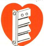
The heart of the Waterfilm Boiler is the zig-zag shaped water tube.
