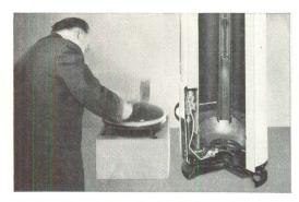
**DIAMOND-TOUGH GLASS** surface of the bottom head of a *Permaglas* Water Heater tank withstands repeated blows from a wooden mallet without cracking or chipping. Blurred hand and mallet show the force of impact.
