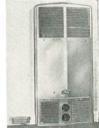
Fitting into any exterior wall between studs, with the Lundstrum vent on the outside wall, they require only one utility connection, to the gas line. Three packaged accessory kits include flue and air intake terminals of lengths to meet the requirements of all types of construction. Saf-Aire heaters are automatically controlled by a floor level thermostat or a manual control. Model 14 measures only 18 in. wide by 24 in. high. Model 20 is 18 in. wide by 38½ in. high.
