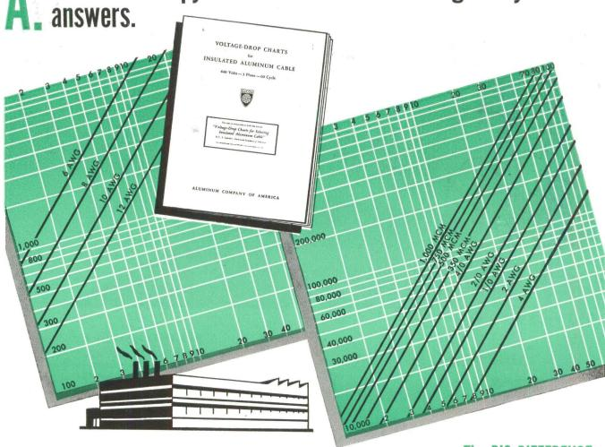
They're worked out here for you—the charts that enable you to determine and specify Alcoa Aluminum Conductor sizes of wire and cable for power and light distribution systems.
