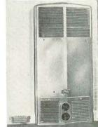
Fitting into any exterior wall between studs, with the Lundstrum vent on the outside wall, they require only one utility connection, to the gas line. Three packaged accessory kits include flue and air intake terminals of lengths to meet the requirements of all types of construction. Saf-Aire heaters are automatically controlled by a floor level thermostat or a manual control. Model 14 measures only 18 in. wide by 24 in, high. Model 20 is 18 in, wide by 381/2 in, high.
