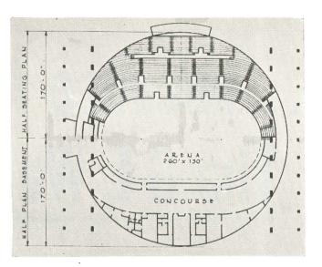
will support the thin shell barrel roof. Alternate arch roof designs were made for concrete and steel. Bidding showed that concrete here had a slight dollars-and-cents-edge, and a handsdown victory on the score of speed. Sherlock, Smith & Adams, Inc., Alabama architectural and engineering firm, designed the new coliseum, with New York engineers, Ammann & Whitney, acting as consultants for the roof and supporting structure. J. A. Jones Construction Co., of Atlanta, Ga. is builder.
