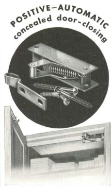
Win-Dor Snuggers and Top-Closers work so well, are installed so easily and cost so little that you can detail them for all cabinet, cupboard and closet doors. These little automatic "hands" actually reach out, grab the door and close it without rebound. Surprising power closes even warped doors and keeps them closed. Surface installation at top, bottom or side. (For complete information see Win-
