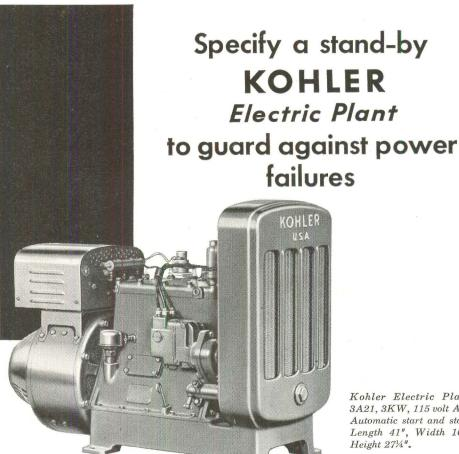
Kohler Electric Plant 3A21, 3KW, 115 volt AC. Automatic start and stop. Length 41", Width 16", Height 271/4".
