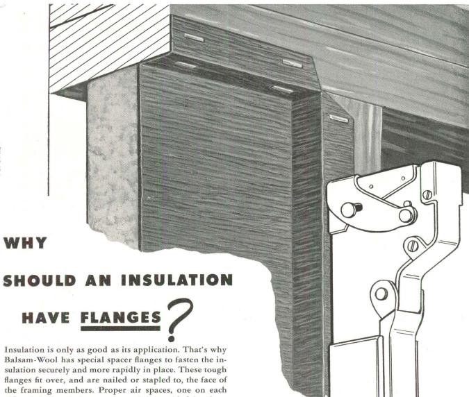
side of the insulating mat, are also provided by these flanges. The result: a sealed, tight, foolproof application for maximum Balsam-Wool insulating efficiency!
