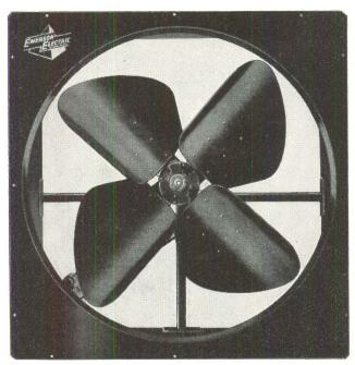
Three sizes: 36-, 42-, and 48-inch, exhausting up to 19,350 CFM. Sleevebearing horizontal discharge type for wall, or for ceiling installation with canvas plenum chamber and automatic shutters. Also ball-bearing vertical discharge type for ceiling installation with automatic shutters.
