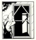
1. NAIL FRAME IN ROUGH OPENING 2. SLIP SASH INTO PLACE
