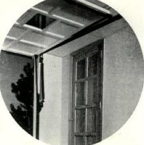
Inside view of Overmatic garage door when "it's up and over." Only 2 inches of overhead clearance required—far less than needed by most overhead doors. Note simplicity of operating hardware. Overmatic can be installed within  $3\frac{1}{2}$  inches of house door in side wall.
