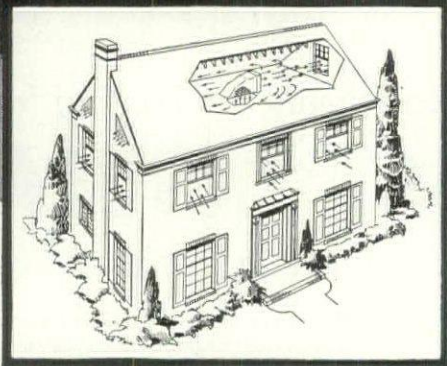
Horizontal-discharge fan installed over ceiling opening, with automatic shutters, and canvas plenum chamber.
