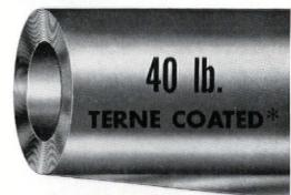
\*Each 435 sq. ft. of copper-bearing steel base plate is hot-dip coated with 40 lbs. of tin and lead alloy (terne coating).
