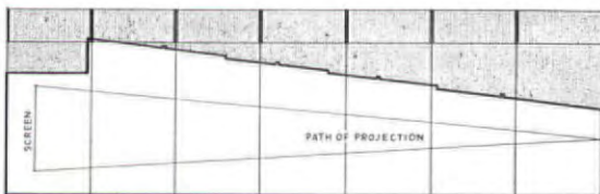
Longitudinal section shows how height of auditorium increases toward screen in keeping with the increasing size of the projection beam.
