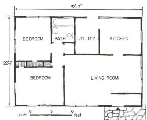
Plan for the T-190 has approximately 750 sq. ft. of living area. Exterior panels for these and other imported models are all insulated for the Temperate Zone (covering most of the U.S).
