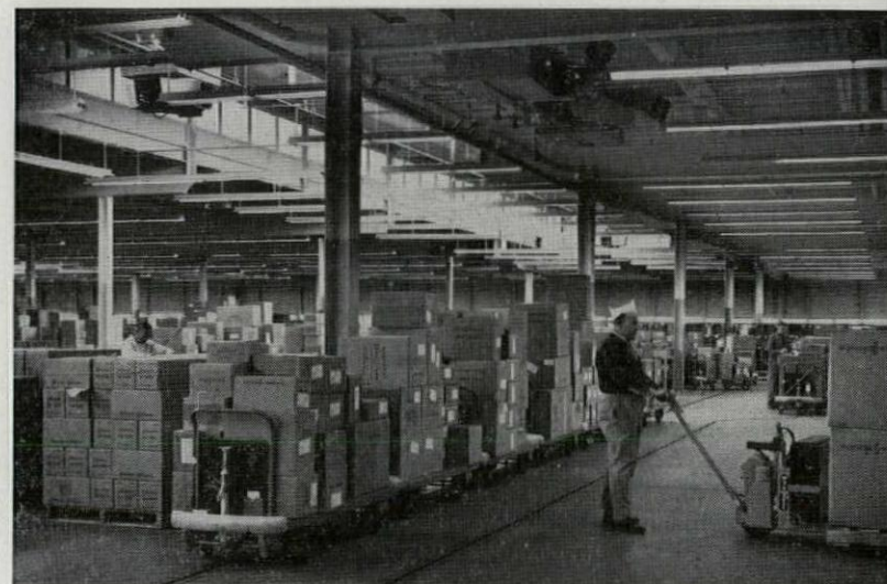
MATERIALS HANDLING is facilitated by drag line trucks which pick up boxed merchandise and deliver it to outgoing rail and truck docks.
