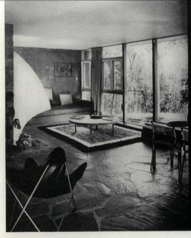
The hooded fireplace draws well and is visible from any point in the living wing. The white concrete hood was built up on metal lath and shaped reinforcing rods anchored into the brick chimney.
