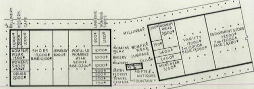
SHADED COLONNADE is created by arcading all storefronts 15 ft. back from column line. This permits each tenant to construct the front according to his individual needs, while the rhythmic line of columns gives architectural unity to the building group as a whole. Gruen calls this a "frame substantial enough to show after the individual pictures are in."
