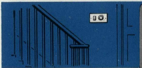
1 Master selector switch in front entrance hall can provide over-all control of lights and outlets.
