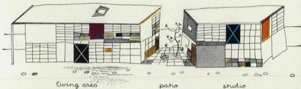
Diagram by Eames shows flexibility of frame, many ways of rearranging facade of patterns
