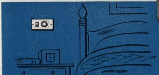
2 Master selector switch in master bedroom can be wired to control fans, coffee makers, and lights right from bedside.
