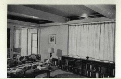
Cove in living room shows how heating and cooling coils are exposed through house. All ceiling, wall, and floor surfaces (under carpet) are reflective, including drapes.
