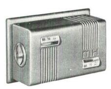
Hospital Thermostat with "Nite-Glowing Dials" — first thermostat ever designed specifically for hospital needs. Luminous dials glow in the dark and are easy to read without lights. No electrical connections required. Magnified indicators. New speed-set control knob, camouflaged against tampering. Simplified design eliminates frequent adjustment. Check here for 12-page booklet on hospital temperature control.
