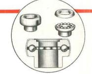
Exclusive Full-Jeweled Ball Bearing assembly consists of a movable and fixed raceway. When lateral thrust occurs, the movable raceway transmits the force directly to the bearings, which, in turn, are held firmly by the fixed raceway. Thus, the weight of the door is supported both laterally and vertically on ball bearings.
