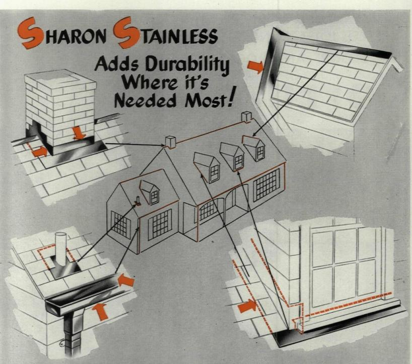
Architects and builders have long been concerned over the "critical areas" — the valleys, ridges, flashing, and gutters that fail under the normal attacks of the weather. The use of stainless steel in these areas has proved to be a desirable improvement. Stainless strongly resists rust and corrosion, making it ideal for ocean front or industrial areas. Stainless has an extremely low coefficient of expansion — tight joints stay tight. There is no excess
