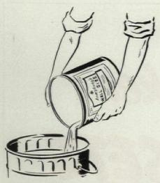
Old plaster. The only preparation needed for bare, unpainted plaster is treatment with Wall Size if porous or dusty. Remove paper, oilcloth, or other coverings. Paint should be removed if unsatisfactory for base (see opposite page).
