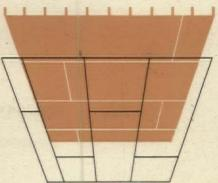
For ceilings longer and wider than 12', apply first layer across the joists, with joints falling between joists. Apply the face layer perpendicular to the first layer, with joints overlapping first layer joints at least 10"
