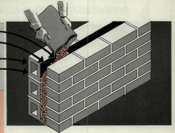
EEE Cavity Wall is a new type of insulated wall which requires no furring or lathing. It can be plastered direct, or interior masonry surfaces may be left exposed.
