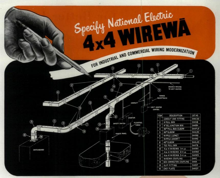
Sketch of a typical 4 x 4 WIREWA installation showing complete flexibility, simplicity and use of fittings.
