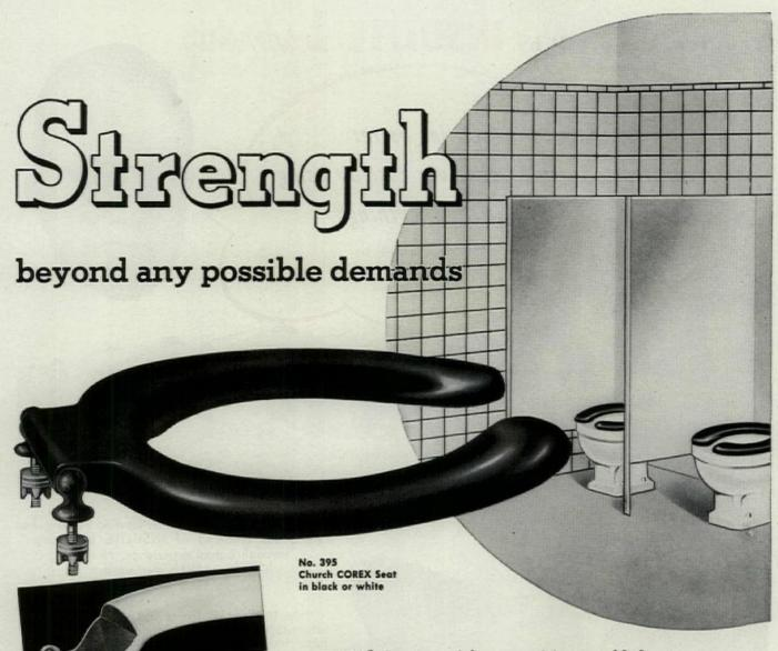
Heavy brass insert imbedded continuously across back and locked into molded core, absorbs any stress, strain or shock. COREX® is a special composition, molded over a core of hardwood fibrous chips, under tons of pressure, into a homogenous unit whose toughness and resilience defies fracture, cracking, chipping, warping or deterioration.
