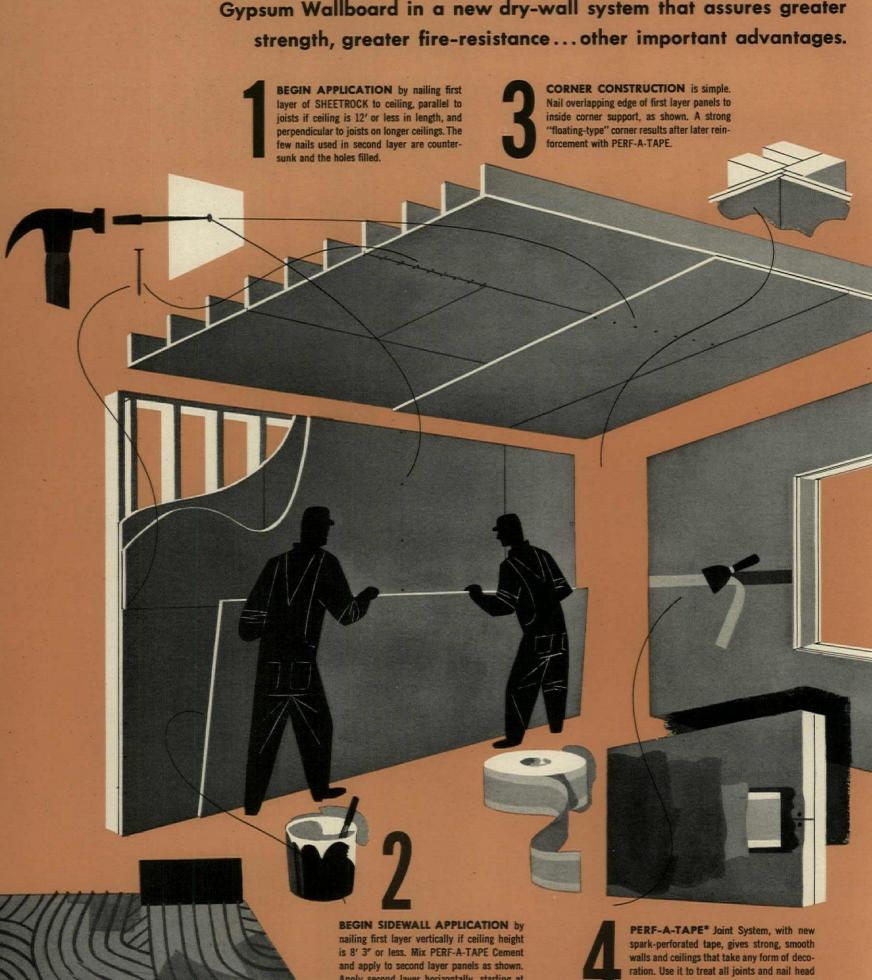
Apply second layer horizontally, starting at ceiling level, for strong cross-lamination.
