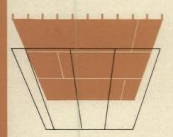
For ceilings not more than 12' wide, but longer than 12', apply the first layer parallel to length of the room, with end joints staggered. Using full-length SHEETROCK Wallboard for face layer, span the width of the room, eliminating end joints.
