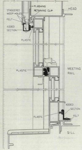
Recommended alterations to windows and spandrel include adding (left, in heavy outline) a section to the bottom of the spandrel which would baffle the weep holes so rain could not be driven directly up into them. This would also make the dam more than 2" deep against pressure differences inside and out. Head gasket of plastic would guard top window, even if left unlocked.
