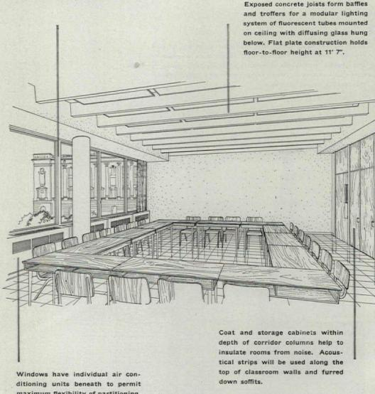
Windows have individual air conditioning units beneath to permit maximum flexibility of partitioning. (Use of fewer units would have saved money but sacrificed some flexibility.) Units are backed by insulation, concrete block and outer spandrel surface of 1/4" ribbed wire glass held in aluminum frame.
