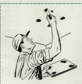
2. Remove the tile. If the paint has not softened, it's safe to install an acoustical ceiling by cement application.
