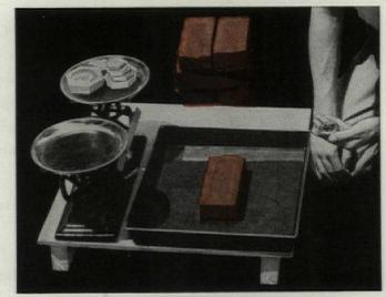
When placed flat in ¼-inch of water for one minute, a brick should gain not more than 20 grams (7/10 oz.)
