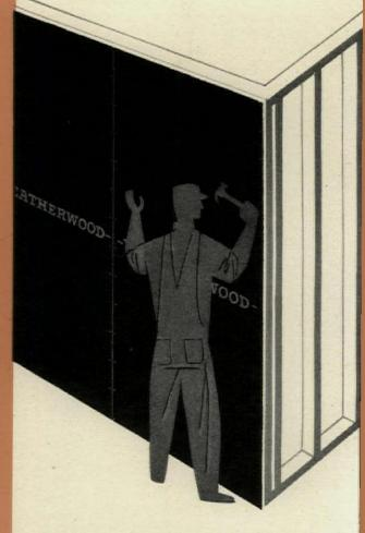
Save up to \$50 a house on framing alone with 4-foot wide, \(\frac{32}{32}\)" thick Weatherwood Insulating Sheathing, FHA-accepted (†) for use without corner bracing. Each board ties 4 studs together, producing firm, rigid walls with greater bracing strength than ordinary horizontal wood sheathing.
