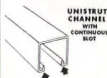
1 WEDGE SHAPED TURNED EDGES TO TAKE SERRATED GROOVES OF UNISTRUT NUT.
