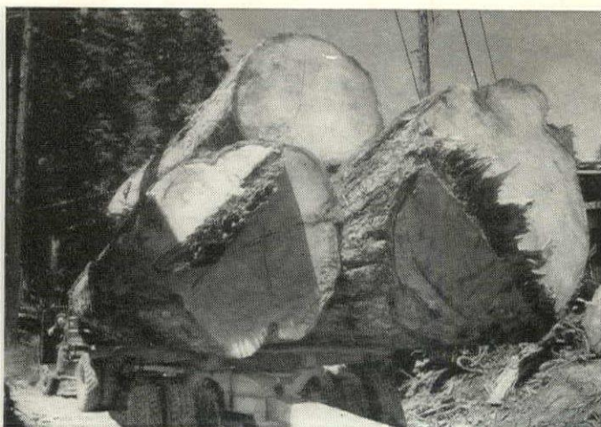
Loads weighing up to 125 tons are carried in one trip on mammoth Weyerhaeuser truck units. Some have two trailers in tandem, making a carrier 100 feet long.
