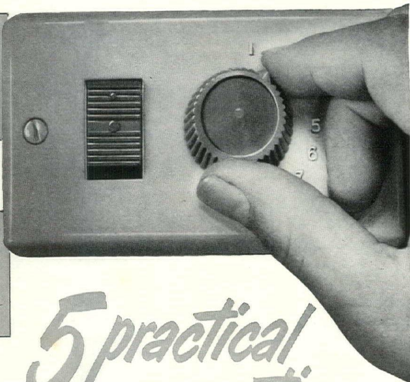
2 Master selector switch in master bedroom can be wired to control fans, coffee makers, and lights right from bedside.
