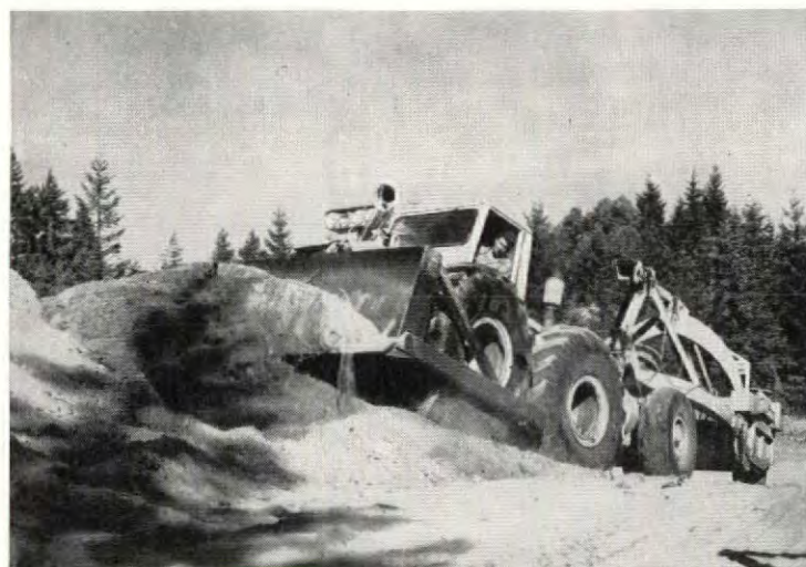
LaPierre's newest piece of heavy equipment is this big $39,500 Tornadoizer with which he clears and rough-grades his own land. It cruises at 14 mph.
