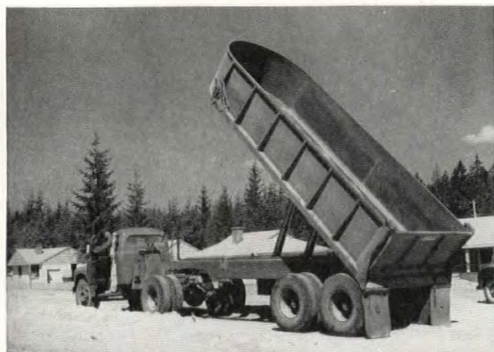
Another item in the builder's $200,000 collection of machinery: hydraulically-operated 17 cu. yd. dump trucks used for hauling gravel, sand and earth.
