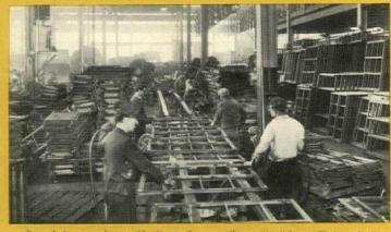
One of the several assembly lines where ventilators are "dropped" into their frames, hinges applied, corners "coined" and dressed down smooth.
