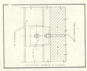
Method employed for attaching channels to old structure. The special slotted clips permitted adjustment where the old wall was out-of-line. Building was first stripped of all projections beyond pilasters, and stone at window ledge levels was cut so that channels could run continuously.
