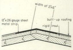
Ridge detail: 4-ply built-up roof
