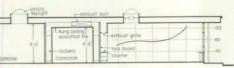
Shift to prefabricated plastic skylights combined good light distribution with economical flat-roof construction.
