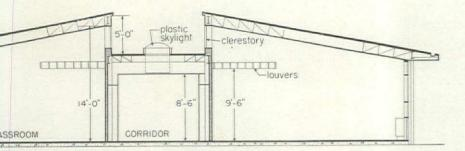
Original scheme for bilateral lighting complicated construction, formed a snow-pocket over the double-loaded corridor.
