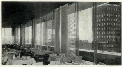
Architects Larson & McLaren, Minneapolis, used *Thermopane* all the way up to the ceiling in the Daylight Wall of the Sky Room of The Dayton Company, Minneapolis. Any non-transparent material would have created an optical barrier. As it is, the ceiling line merges with the sky. This promotes a sense of great expansion, of roominess. It is an architectural device which can make any room seem larger than it is.
