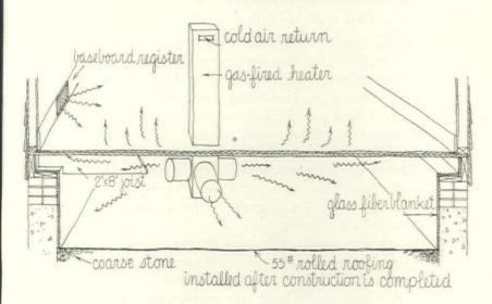
Most economical installation is with the furnace in center of house as shown here. Cost is only slightly higher with furnace in utility room at side of house, with 10' or more of duct carrying air part way across crawl space.
