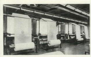
\$1500 Saved Here. This unique inspection method uses 24 forty-watt Sylvania fluorescent tubes and a luminous panel. Mill engineers estimate this Sylvania-designed unit provides a saving of \$1500 per year.
