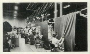
Inspection speeded here. Excellent use is made of the flexibility of Sylvania Fixtures. Hung at an angle over the cloth they eliminate need for slow, costly hand portable droplights and greatly speed inspection. Another big saving with Sylvania.
