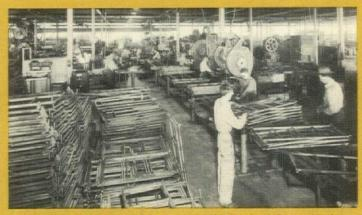
Ventilating portions of the windows are assembled first, by air hammer riveting and automatic flash welding.
