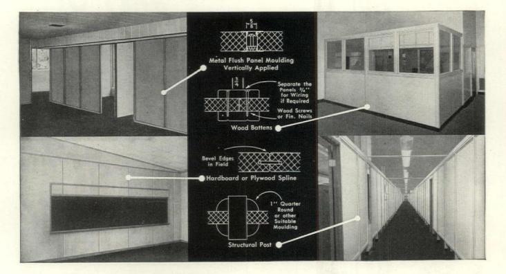
Each 4' wide Cemesto Insulating Structural Panel is a *complete* partition unit that needs no finishing! Used with new flush-type steel accessories or wood millwork, Cemesto Panels simplify and speed erection. They build strong, durable, handsome dwarf, free-standing or full partitions . . . at remarkable savings in time, labor, materials!
