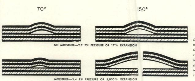
Difference in force between dry and wet blister is shown graphically in these diagrams. Top two show the expansion caused by heating a dry blister. Bottom two show how much greater is expansion of a damp blister heated to same temperature. (See also sketch at bottom of page.)
