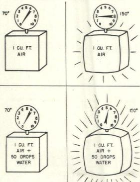
A cubic foot of dry air heated from 70° to 150° generates considerable pressure (sketch left), but if it is damp air it generates much more pressure.
