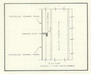
Vertical section through porcelain enameled panels showing attachment detail. The furring strips are welded directly to 4-inch light structural channels and are continuous at each horizontal joint. Each individual panel is a self-supported unit.
