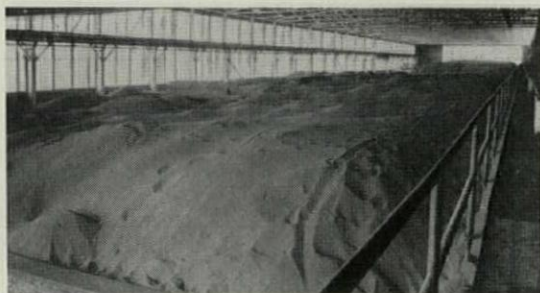
This straight-line foundry for Ford and V-8 Mercury engines composes a vast materials handling problem. Sand (to form the molds) goes in one end; hot metal meets it halfway down the line. Photo above is 20' high pile of sand, brought in by rail and dropped in conveyors. In photo at right the sand is being dried.
