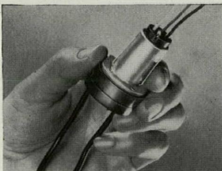
Heart of the 277-volt lighting system is this RR-2 remote-control relay. It will switch up to 5 amperes of fluorescent load. Operates on 24 volts, mounts through ½-inch knockout of outlet box or fixture.
