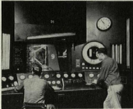
CONTROL ROOM is where testing engineers watch dial gauges, flow meters, switches, indicator light and scales. This one is at the former Dodge Chicago plant. Radial engine can be seen through bulletproof window.
